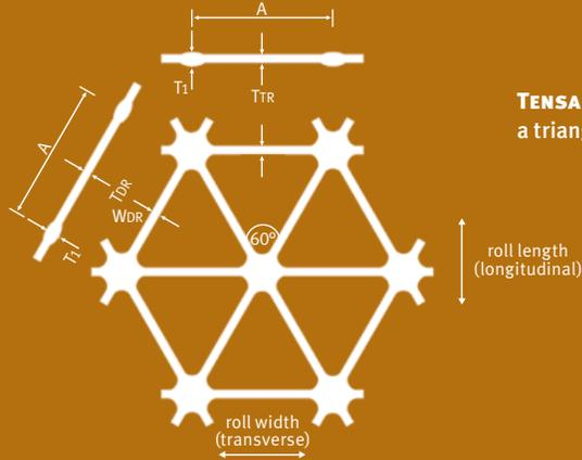
TENSAR® TRIAX® GEOGRIDS have a triangular aperture structure.
