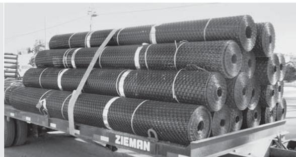
Image 1 Storing the Tensar TriAx Geogrid rolls (horizontally).
