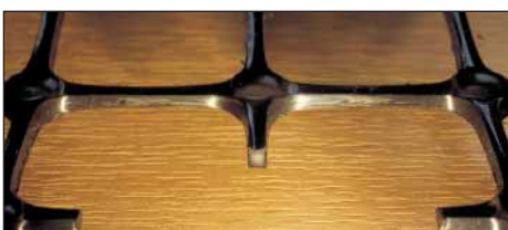
Figure 4a: The importance of the shape of Tensar biaxial geogrid ribs.
