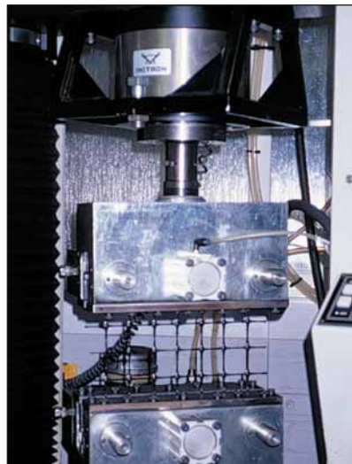
Figure 28: Test arrangement and result for ISO 10319 tensile test on Tensar SS30.
